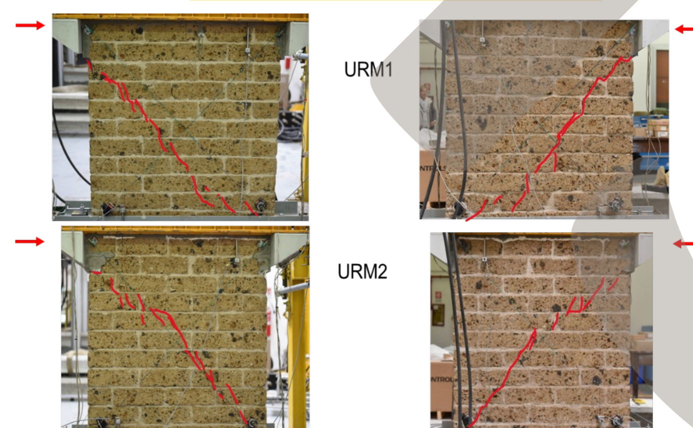
Shear Failure in tuff blocks
