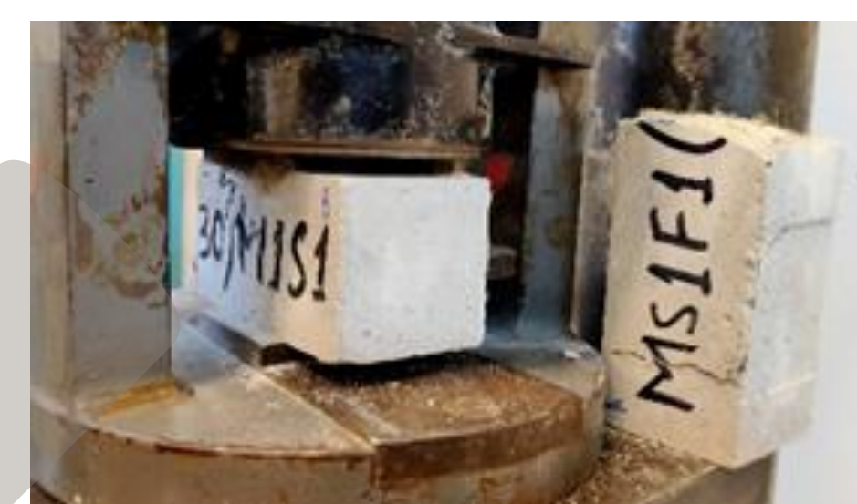
Compressive strength tests: Samples without and with fiber
