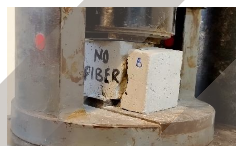
Compressive strength tests: Samples without and with fiber
