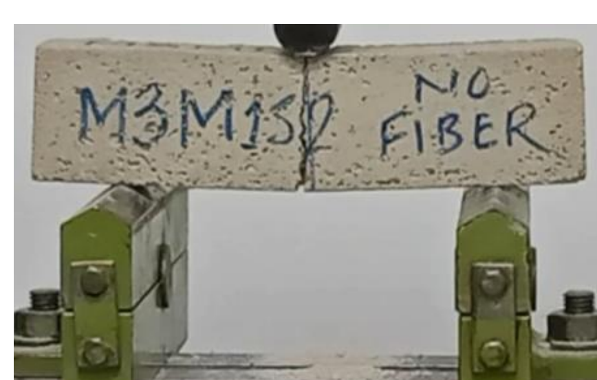
Flexural strength tests: Samples without and with fiber
