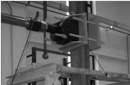
Figure 22. Connection of actuator to the specimen.
