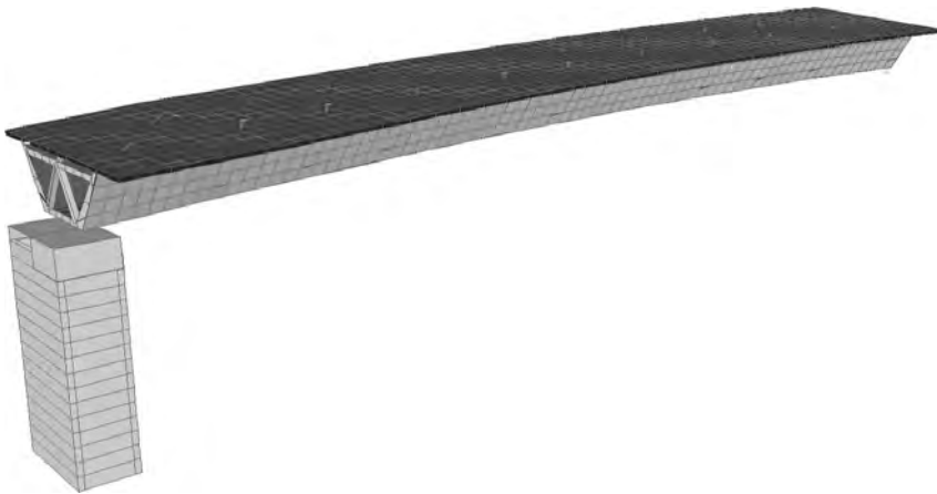
Figure 19. 3D FE model used for dynamic analysis purposes.
