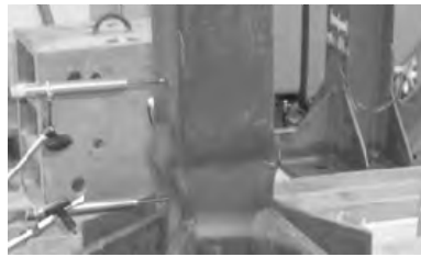
Figure 32. Failure mechanism of SHS160x160x6.3 specimen under cyclic loading.
