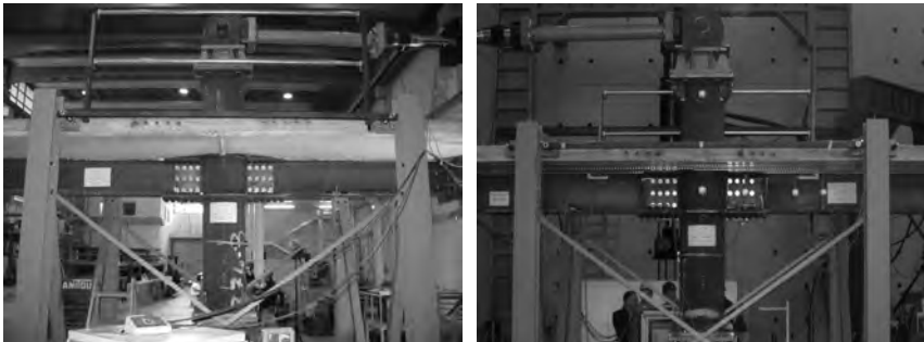
Figure 8. Bolted beam-to-column specimens a) slab with electro-welded lattice girders, b) slab with profiled steel sheeting.
