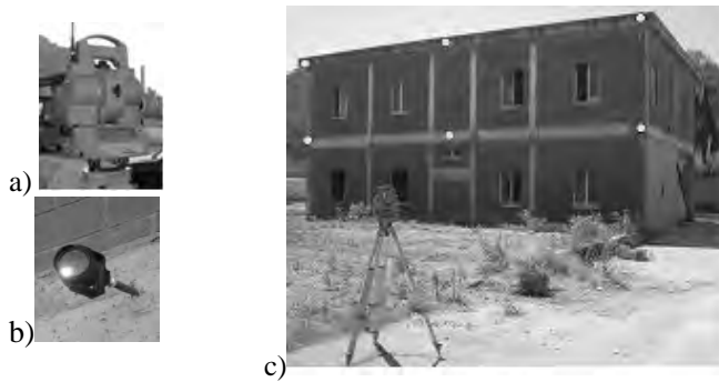
Figure 8. Location of station and reflecting targets.
