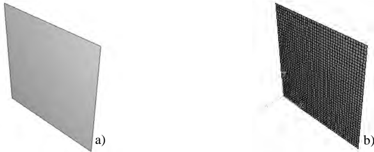
Figure 60. The numerical model of a SPSW (a) and the used mesh (b).
