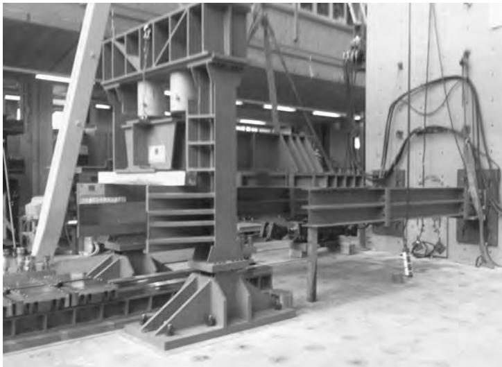
Figure 30. Isolator testing machine at the University of Basilicata in Potenza.
