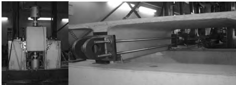
Figure 19. Details of testing of structural connection.
