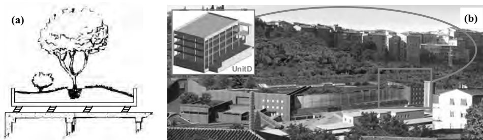
Figure 34. (a) The concept of roof-garden TMD; (b) the application to a building in Siena.
