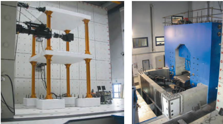
Figure 4. Reaction wall (left) and bearing tester system (right) of the TREES Lab, Eucentre, Pavia.
