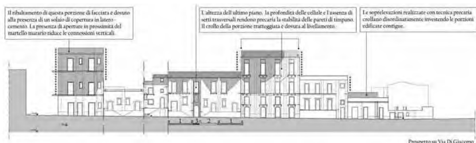
Figure 1. Seismic scenario of a building aggregate in Catania.
