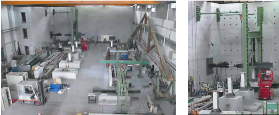
Figure 5. Aerial view (left) and large reaction wall (right) of the MST Lab, Trento.
