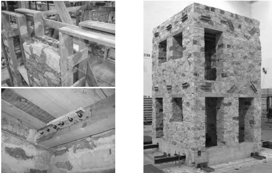
Figure 20. Construction, detail and global view of a model stone masonry building tested on shaking table (Mazzon et al., 2009).
