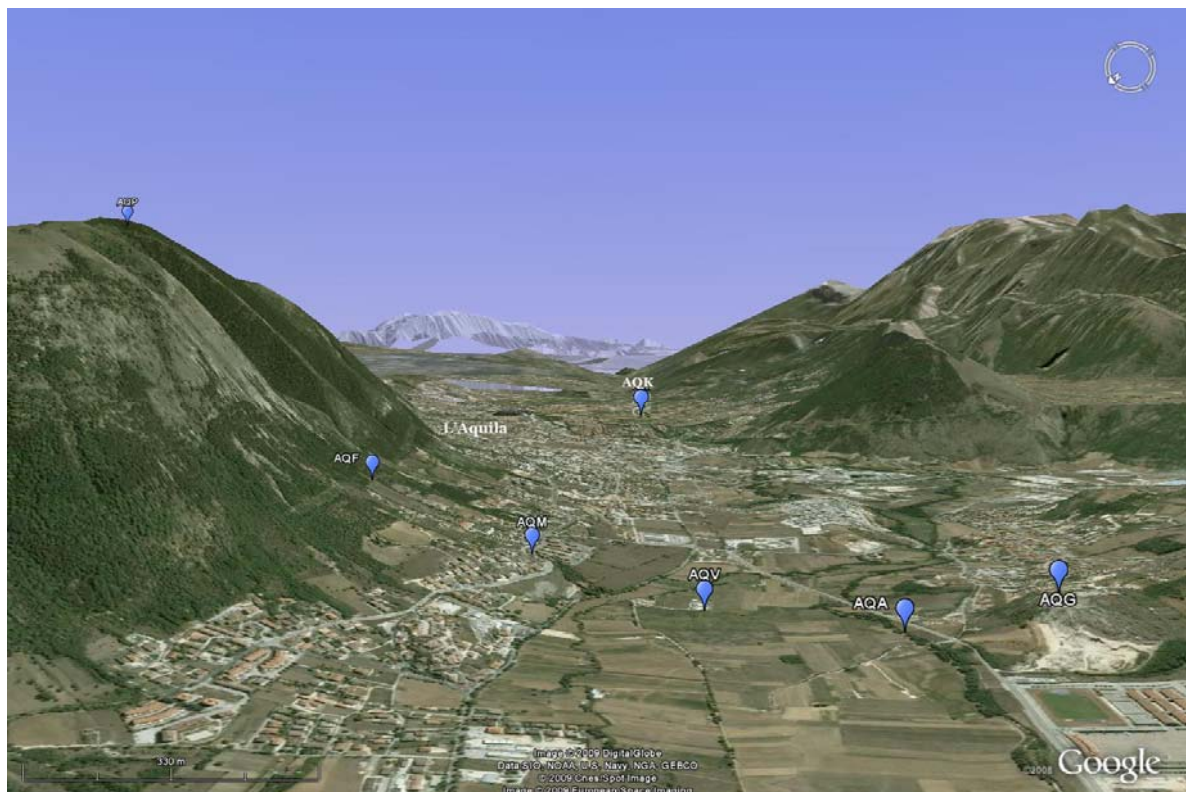
Figure 2. General view of the Aterno valley and bordering mountains showing the location of the strong-motion stations belonging to the DPC array (AQG, AQA, AQV, AQM, AQF, AQP); in the background the station AQK in the city of L'Aquila (vertical scale enlarged 2x).
