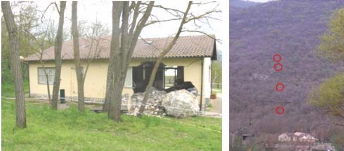
Figure 57. Block detached from a rock cliff above the Stiffe Caves (left). Impact marks (on the right) individuated by Scott Kieffer and Edward Button (GEER Working Group 2009).
