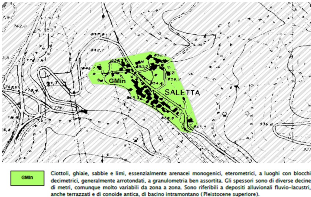
Figure 5.65. Geological setting of Saletta hamlet, retrieved from the Level 1 Microzonation map of Amatrice (Regione Lazio, 2016).
