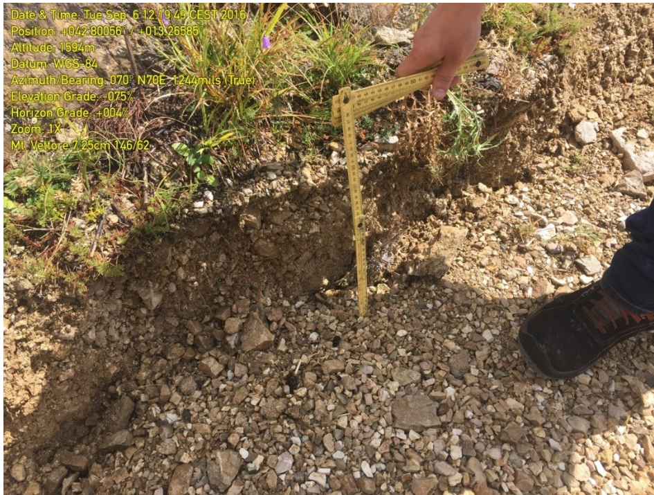
Figure 2.19i. Mt. Vettore fault Site 7 at a WGS84 ellipsoid elevation of 1594 m. The normal fault displacement at this site was 25 cm down toward the west. (Latitude and Longitude are annotated on the image).
